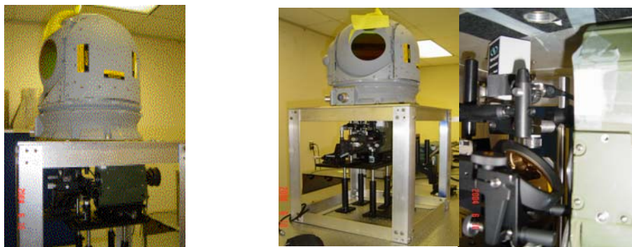
Figure 8.4 IRST with MELIOS & laser path integration
